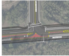
Continuous Green-T One major street direction of travel continues through the intersection without stopping. All other street lanes would stop at the intersection with a traffic signal.
