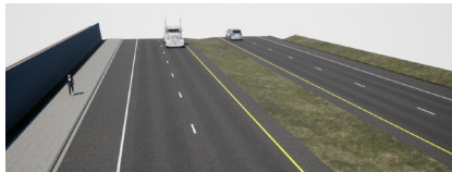
4-Lane + Median with Attached Pathway
