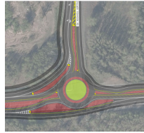
Roundabout A circular intersection where vehicles move counterclockwise around a central island. Vehicles within the roundabout have right-of-way, and those entering must yield.
