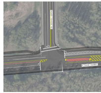
Traditional Traffic Signal An intersection where movement has dedicated lanes for efficient flow (e.g. an additional lane for right and left turns). A standard traffic signal would correspond to individual lanes to control movements.
