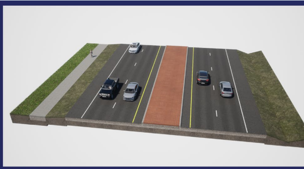
Raised Median with Turn Lanes
